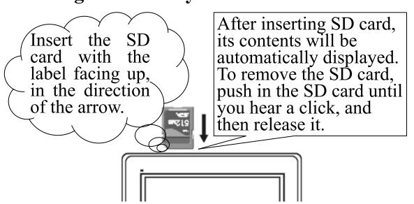
Note: Do not remove a SD card or turn off the device while transferring data, as data might be damaged.
