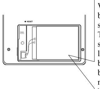
While installing the battery, the battery should be inserted flat. The side with wires should be facing the left. While inserting the battery pin into the battery point of the battery pin should be upward.
