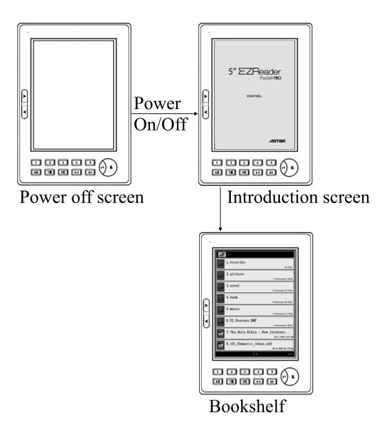
To switch off, press and hold the on/off button for a few seconds.
