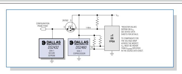
Figure 6. Configuration settings can be written to the DS2432 by adding a single transistor and a configuration probe point.
