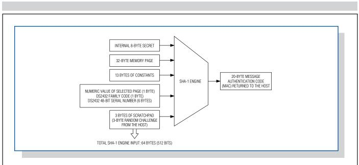
Figure 8. Specific DS2432 SHA-1 engine input data is shown for the challenge-and-response authentication MAC.
