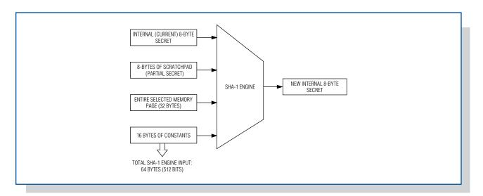
Figure 10. Input data is used for a device-performed secret computation; the lower 8 bytes of the 20-byte MAC result become the new secret.
