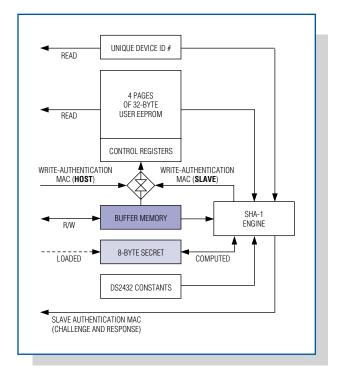
Figure 7. All major data elements and data-flow paths are shown for the DS2432 SHA-1 secure memory data-flow model.
