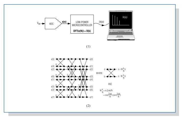
Figure 1. The spectrum of an input voltage is calculated using an FFT application. (See article inside, page 9.) Figure 2. A butterfly computation is used to perform an FFT for N = 8. (See article inside, page 10.)
