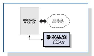
Figure 4. A reference design is authenticated through use of the DS2432.
