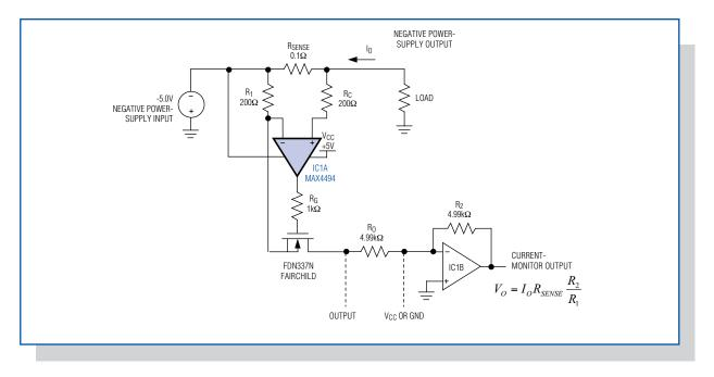
Figure 1. This current-sensing circuit monitors a negative power supply and provides a positive output voltage proportional to the load current.
