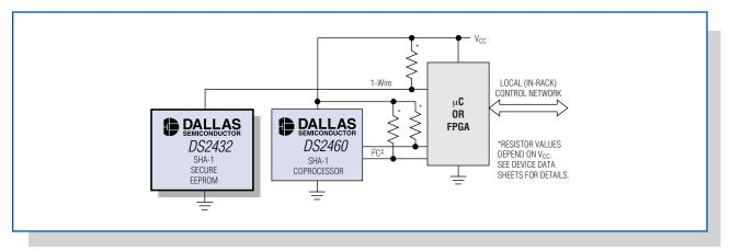
Figure 3. A DS2432 EEPROM device is implemented in a typical board environment through use of a free I/O pin and a pullup resistor.
