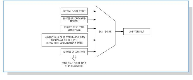
Figure 9. SHA-1 engine input data is used to compute a write-access authentication MAC.
