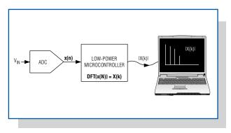
Figure 1. The spectrum of an input voltage is calculated using an FFT application.
