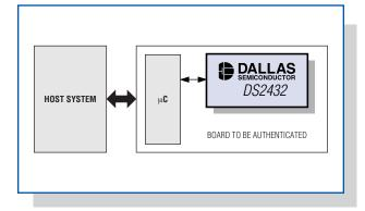
Figure 5. This HW authentication example shows a cloned circuit board with an exact copy of the firmware/FPGA configuration or a cloned system host.
