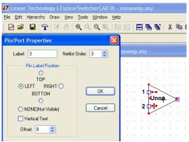
In the Label box of the Pin/Port Properties dialog box enter the label that matches the schematic oaBlock.asc.
