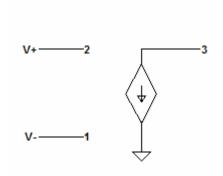
This is what a schematic of the subcircuit would look like. "g1" is a linear voltage controlled current source with pins of <+node><-node><+controlling node><-controlling node>< gain>. Now when the symbol is made the "netlist order" of the pins will be Inverting Input (pin 1), Non-Inverting Input (pin 2), Output (pin 3).
