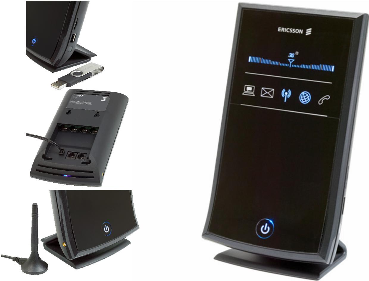
The Ericsson W30/35 Mobile Broadband Router utilises an existing 2G/EDGE or 3G/HSPA mobile network to provide phone, broadband and fax services to enterprise and small businesses, without the need for a fixed telephone line or access to a cable network. Simply insert a SIM card into the Mobile Broadband Router, plug it into a power point and the device is ready for use.
