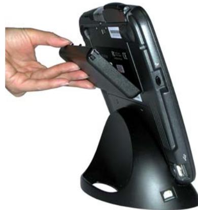
To attach the battery pack, align (and insert) the two lower tabs on the external battery pack with the two grooves in the designated area (Figure 2). After insertion into the grooves, squeeze the two tabs at the sides of the battery pack while pushing it flat against the rear surface of the WebDT 375. Release the two tabs and verify that the battery pack is secure and flush against the WebDT 375.
