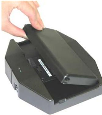
**Figure 4:** Insertion of WebDT 375 External Battery Pack.
