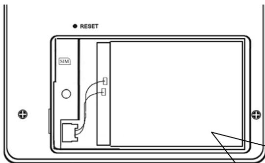
While installing the battery, the battery should be inserted flat. The side with wires should be facing the left. While inserting the battery pin into the battery socket, the metal point of the battery pin should be upward.
