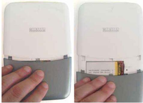
You can easily access the battery and the reset hole of your Cybook Opus. The battery and the reset hole are located in the back of the unit behind a removable sliding part of the external housing. No screws are needed to access this compartment.
