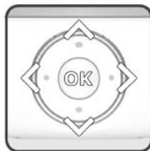
The navigation control is a 5 way control button (left, right, up, down) plus a central validation key. The navigation button is used to turn pages (right, left) to move a selection on the screen (up, down, right,
