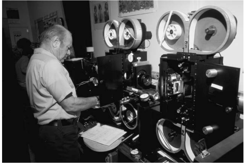
Making a composite image for Star Wars on the ILM-rebuilt optical printer originally created for Columbia's Marooned (1969).
