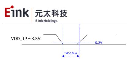
Note : During power off, the VDD\_TP must be less than 0.5V for at least 10us to make sure the touch controller is power off correctly.
