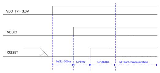
Note: I/F start communication must star after XRESET successfully 300ms. The rising time of VDD\_TP should be less than 1ms. Power signal can't ramp down during power rising cycle.
