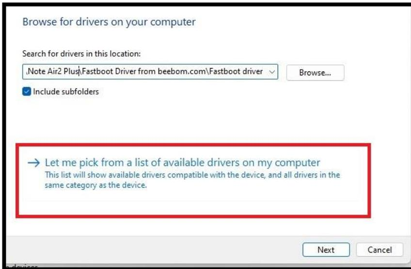
6. Once you have installed the driver, Windows may request a reboot. If Windows prompts you to do so, do this while your Tab Ultra C is still in Bootloader mode. I believe it is necessary to make the driver installation work.
