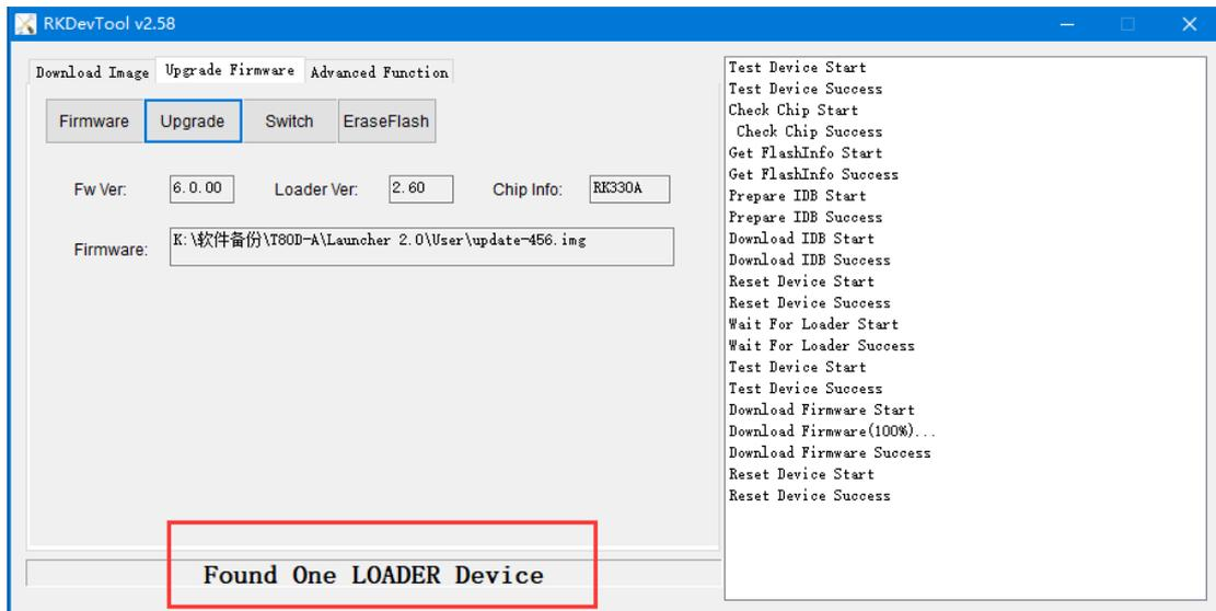
7. When the rooting finished, there will be “Reset Device Success” reminder on the right side of tool. (Please wait the device to restart and no USB cable loose during this time)
