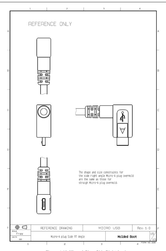
Figure 4-15 Micro-A Plug, Side Right Angle
