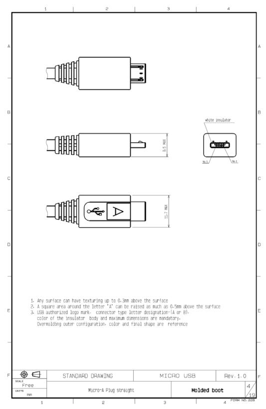
Figure 4-4 Micro-A Plug Overmold, Straight
