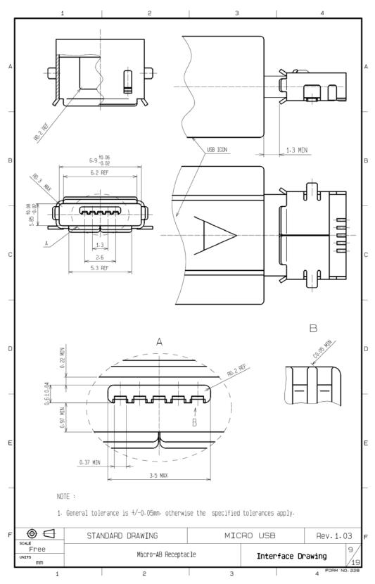
Figure 4-9 Micro-AB receptacle interface
