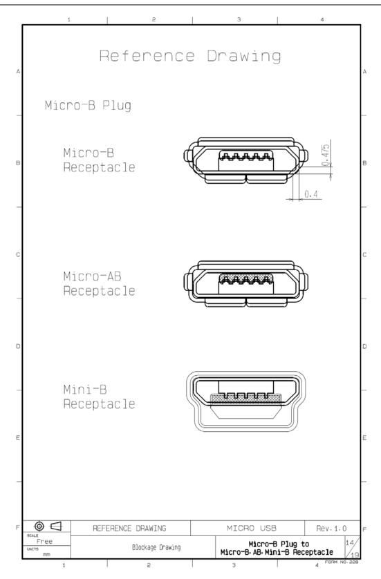
Figure 4-14 Micro-B Plug Blockage
