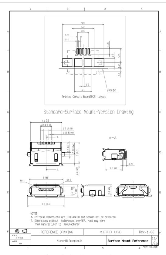
Figure 4-11 Micro-AB Receptacle Design
