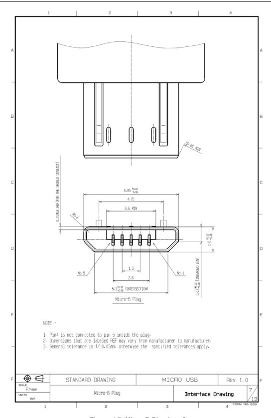
Figure 4-7 Micro-B Plug Interface
