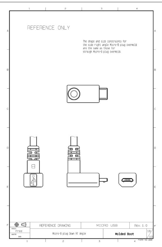
Figure 4-18 Micro-B Plug, Down Right Angle
