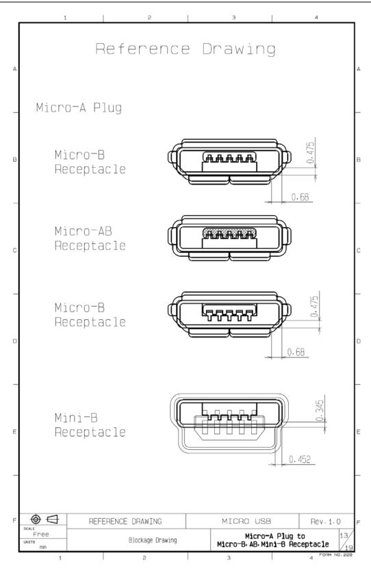
Figure 4-13 Micro-A Plug Blockage
