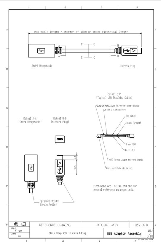
Figure 4-19 Adapter, Standard-A receptacle to Micro-A plug
