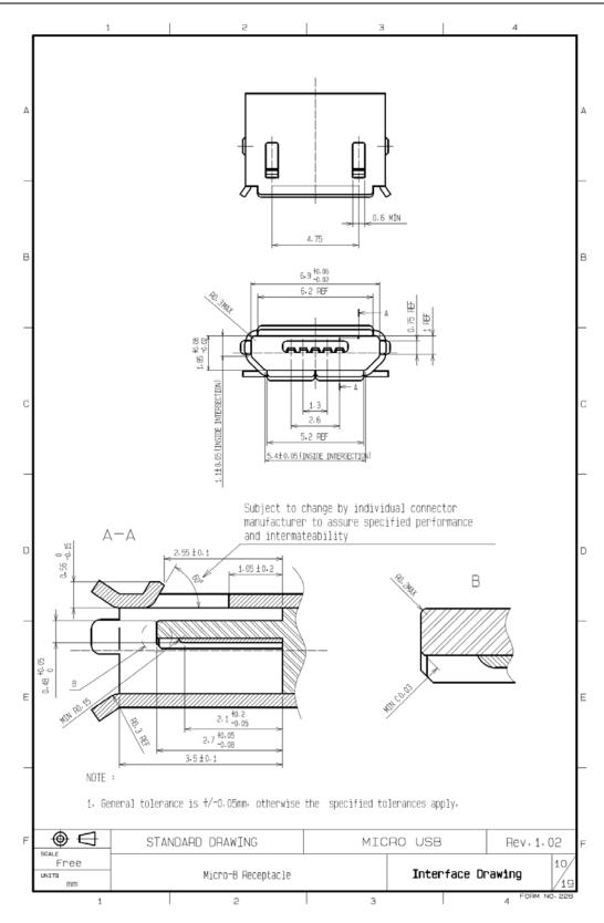
Figure 4-10 Micro-B receptacle interface
