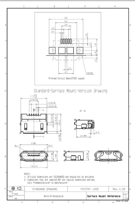
Figure 4-12 Micro-B Receptacle Design
