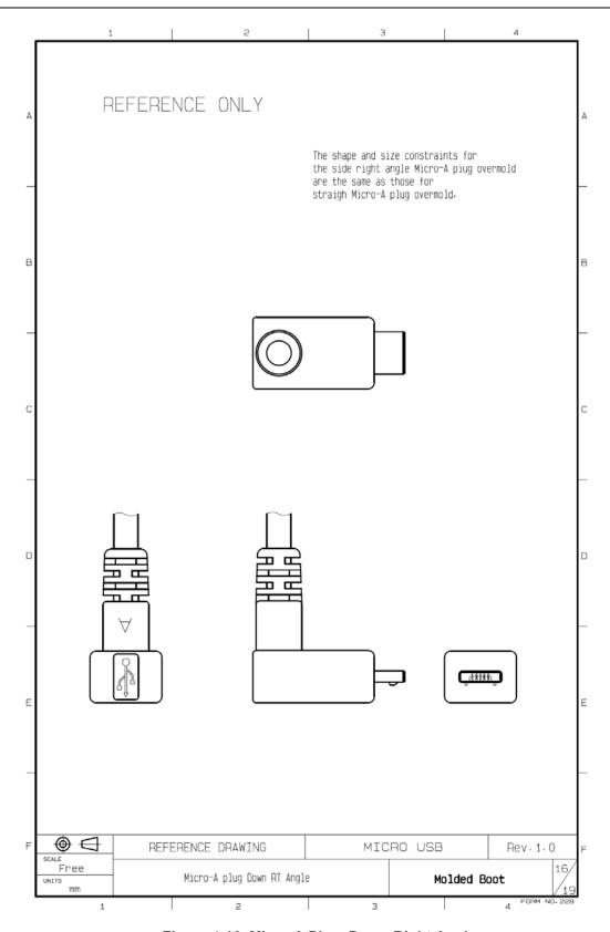
Figure 4-16 Micro-A Plug, Down Right Angle
