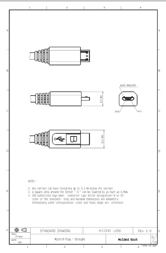
Figure 4-5 Micro-B Plug Overmold, Straight
