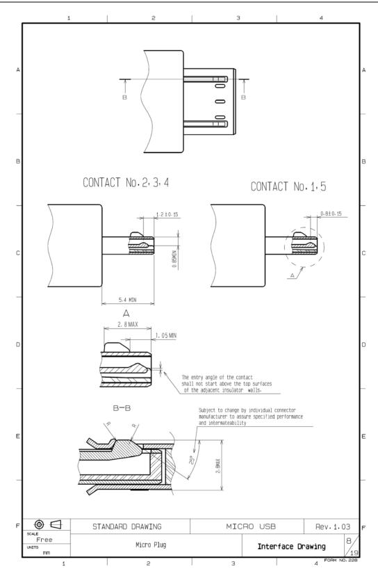
Figure 4-8 Micro-A/B Plug Interface (Cut-section)
