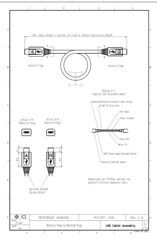
Figure 4-1 Micro-A to Micro-B Cable
