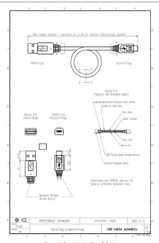
Figure 4-2 Standard-A to Micro-B Cable
