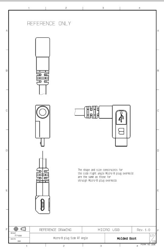
Figure 4-17 Micro-B Plug, Side Right Angle
