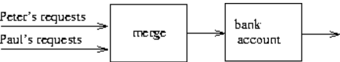
Figure 3.38: A joint bank account, modeled by merging two streams of transaction requests.
