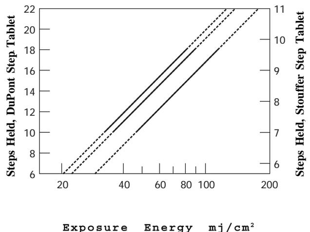
Figure 1: Riston® Film Steps Held vs. Exposure Energy
