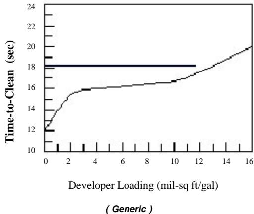
Data was generated with a 38 µm thick film developed in 0.85 wt% Na<sub>2</sub>CO<sub>3</sub>, 2 bar spray pressures. Note the rapid change during initial loading, the conveyor breakpoint should be adjusted accordingly
