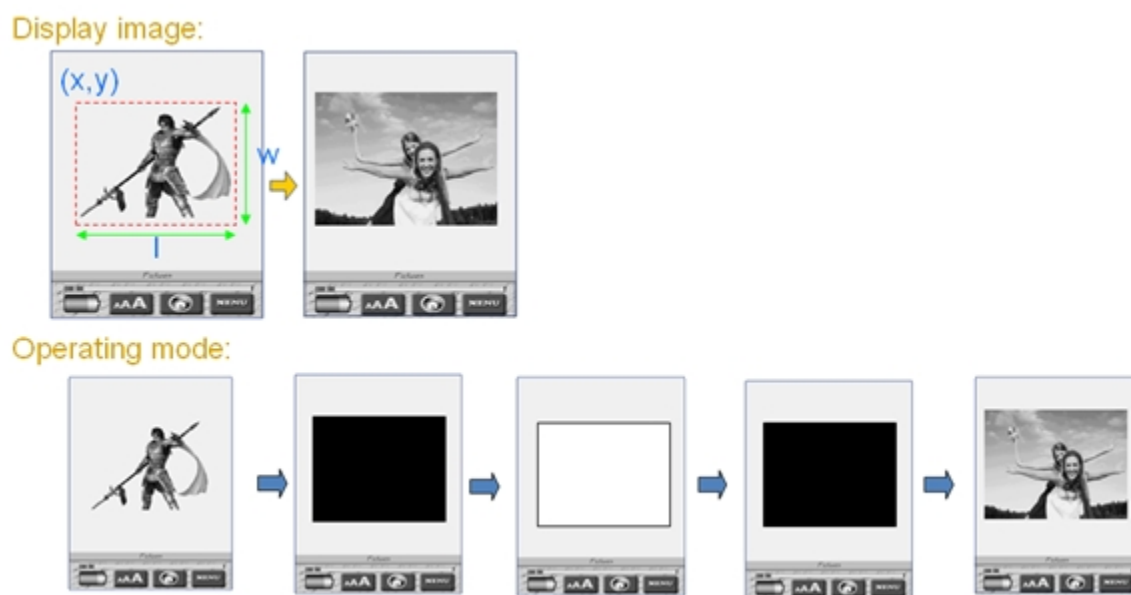
Figure 42-11. The example of screen update with mode 0 waveform
