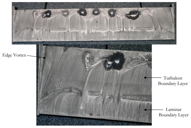
Figure 3.14 - Oilflow Visualisation - Clean Wing Complete and Edge
