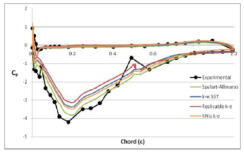
Figure 4.8 - C<sub>P</sub> Plot of Alternate Turbulence Models - Co Rotating SVG Wing
