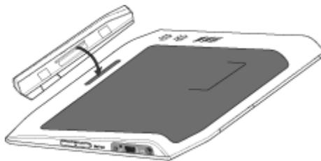
4. Check to make certain that the device is positioned correctly. Magnets will secure the light in place when you let go of it.
